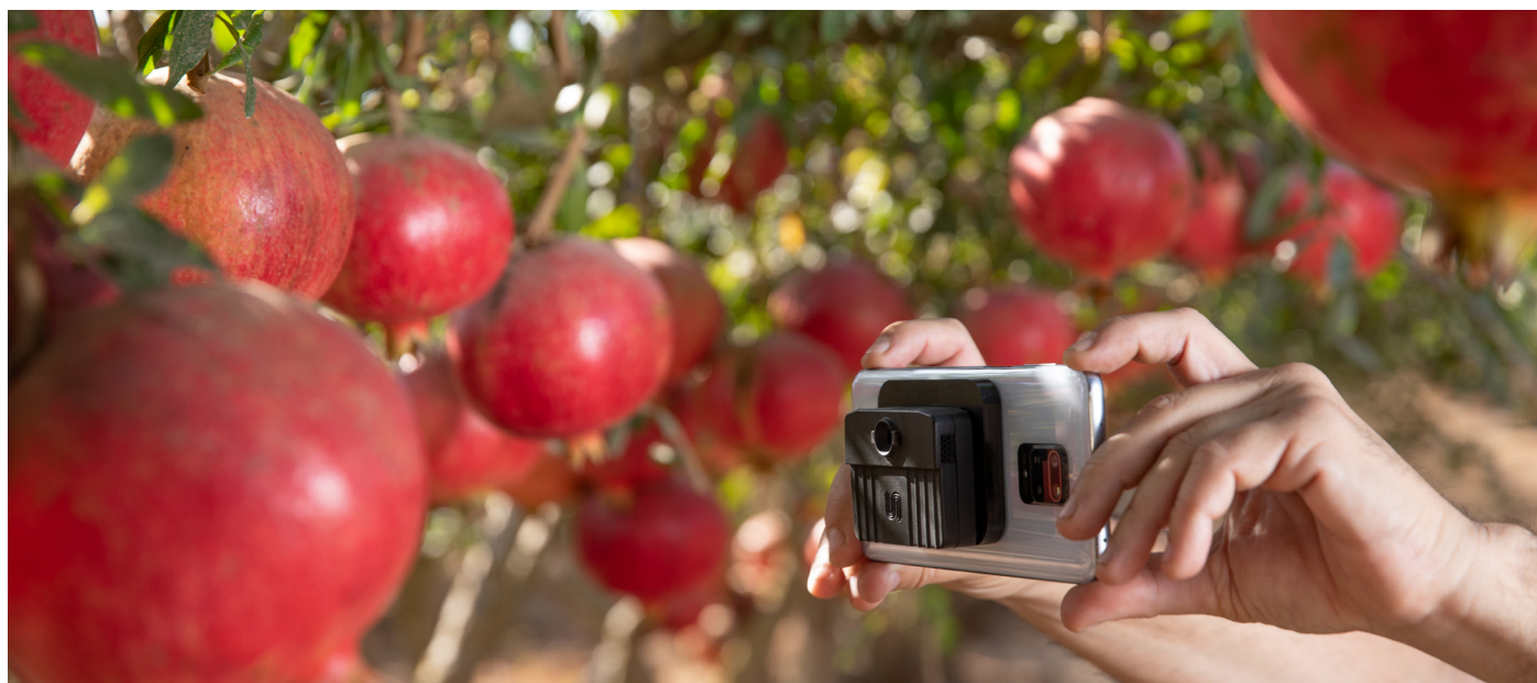
Figure 1: Unispectral Monarch Camera mounted on smart phone for fruit monitoring
