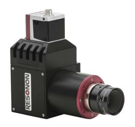
The Pika L is a line-scan hyperspectral camera that covers the visible and near-infrared spectral range (400 – 1000 nm). The Pika L is lightweight and compact, ideal for remote sensing. It can be used with any of Resonon's benchtop, outdoor, and airborne systems, standalone with our software development kit, and integrated into machine vision systems.
