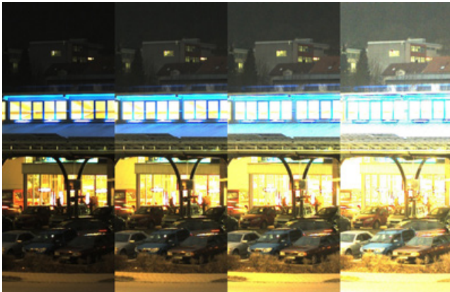
Figure 1 Four extracts of the same night image, which was taken in the evening out of the lab towards a supermarket in Kelheim with a pco.edge 5.5 color sCMOS camera system. The difference between each column is the way how the 16 bit image was scaled to the 8 bit world of the print or the screen, but all versions have been created of the same raw data file. The first column on the left side shows a full scale conversion (value 65536 (16 bit max) -> value 256 (8 bit max) and value 0 (16 bit) -> value 0 (8 bit)), while the column on the right shows a low scale conversion (value 1024 (16 bit low) -> value 256 (8 bit max) and value 0 (16 bit) -> value 0 (8 bit)). The other columns show different conversions in between.
