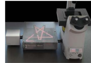
MicAO plugged in between the microscope and the camera, ready to be used.
