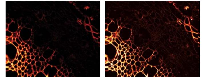
Uncorrected and AO corrected 2-Photon-Excited fluorescence (2PEF) Microscopy - Plant tissue - Drs. Beaufreire, Débarre & Olivier, Ecole Polytechnique, LOB (CNRS-INSERM), France.
