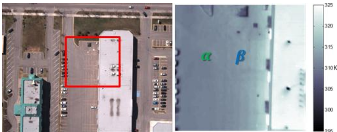
Figure 7 Airborne visible image of the gas release area (left) and infrared broadband image of the target area of interest (right). Areas corresponding to the asphalt pavement and a location near the gas release point are labeled by \alpha and \beta respectively.
