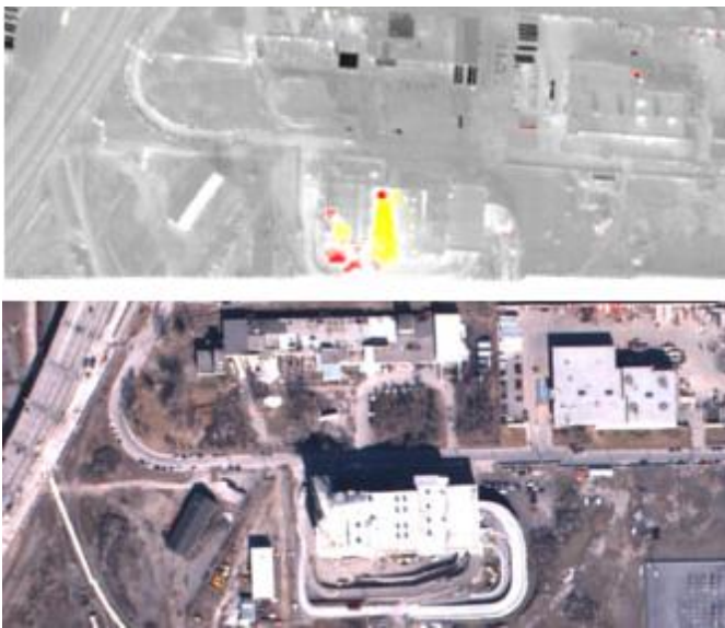
Figure 7 Chemical imaging of water vapor (H 2 O, yellow cloud) and water aerosol cloud (red cloud) from a waste incinerator (top). Visible image (bottom) is shown for comparison purposes.
