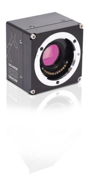
The EXO Tracer is an industrial camera with a fully functional lens control (focus, zoom, aperture). Lens mount is a Micro Four Thirds (MFT) mount. The excellent thermal concept of the EXO qualifies for a operating temperature of up to  $60^{\circ}$ C.
