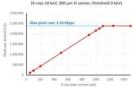
Maximal pixel rate of MiniPIX TPX3
