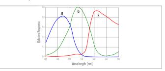
$^{\star}$  Sensor data — excludes camera cover- or IR-cut filter characteristics
