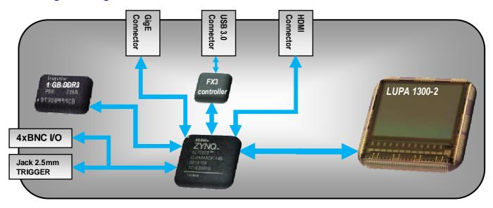
These abilities are used to realize image triggers, lossless compression and as example binarisation of images, on the fly data generation like blobs edge or barycenter coordinates.
