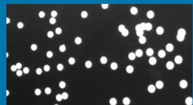
A similar image of the same test beads as above using the pco.edge (@ + 5°C) shows that the offset control of the pco.edge performs efficiently.
