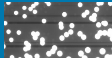
Extract at the boundary of a competitor’s sCMOS camera (@ - 40°C). The image of fluorescent test beads illustrates the issue of reference pixels when illumination falls onto the boundary. The dark bands from the changed offset are clearly visible.
