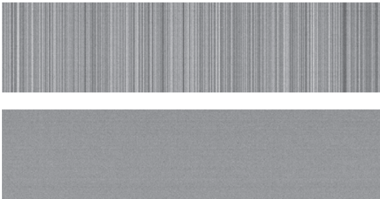
The upper image shows a typical fixed pattern noise in a CMOS image sensor, which is caused by small differences of the column amplifiers of the sensor. The lower image shows the corresponding image of the scientific CMOS pco.edge camera at +5°C sensor temperature with the standard FPGA based calibrated dark image.
